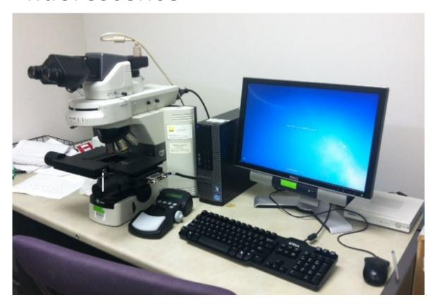
Motorized stage with image stitching software NIS Elements imaging and analysis software
