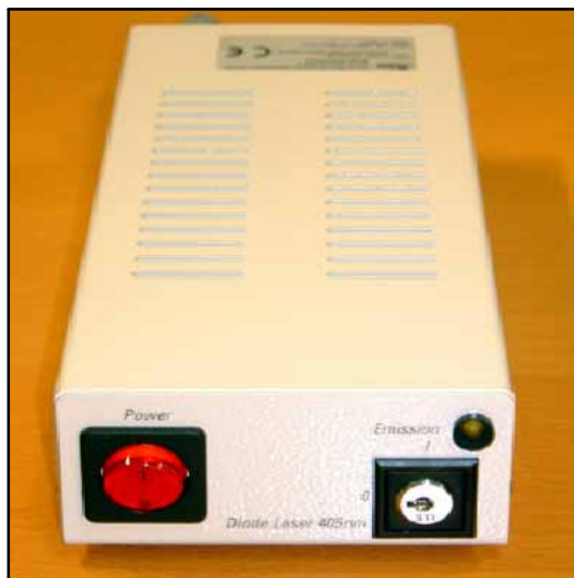
figure8. Detachable-key switch of the external 405-nm Advance laser
