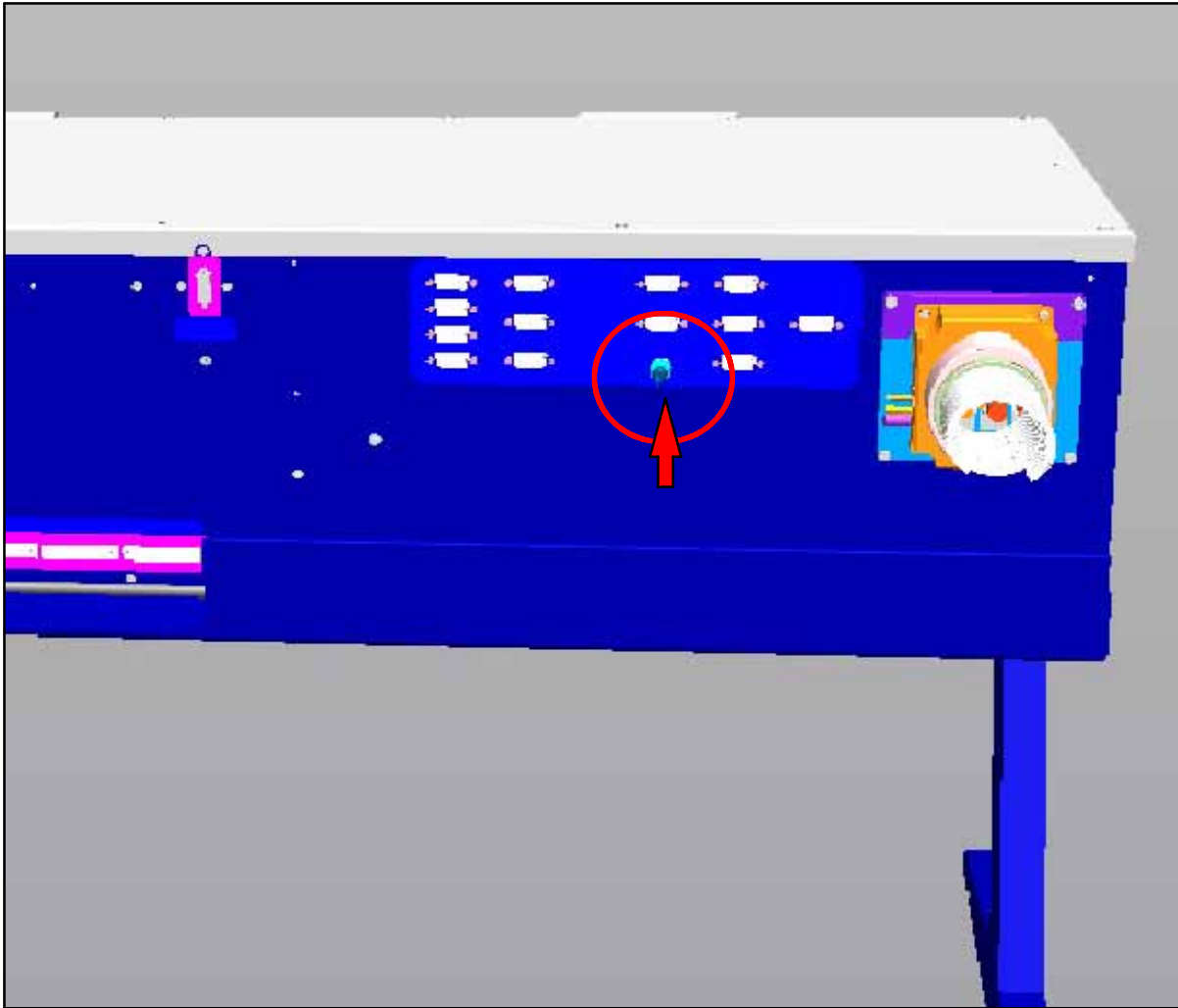
figure11. Position of the remote interlock connector
